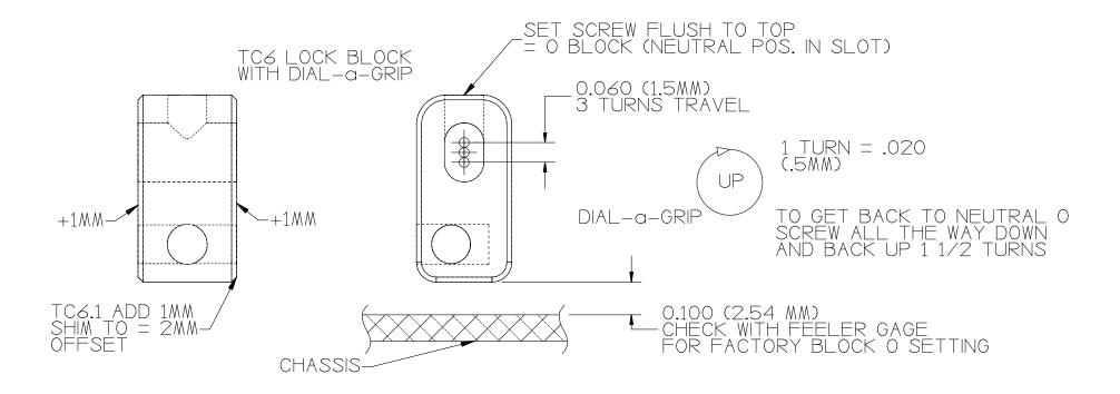
1 FULL TURN OUT ON DIAL-a-GRIP MOUNTED AT B HOLE = AE A3 SETTING TO ADJUST ARM ANGLE - LEAVE ARM PIN LOCKS TIGHT AND LOOSEN BOTH L AND R BLOCK 1/2 TURN ADJUST DIAL-a-GRIP THEN TIGHTEN WHILE PUSHING DOWN TO LOCATE.
